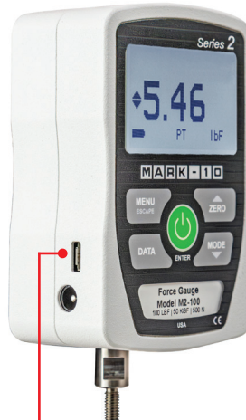
USB port for data communication
